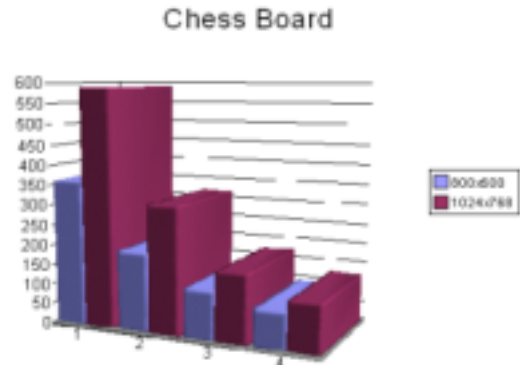
Figure 6: Results of rendering chess.pov on a cluster with varying number of processing slave nodes
